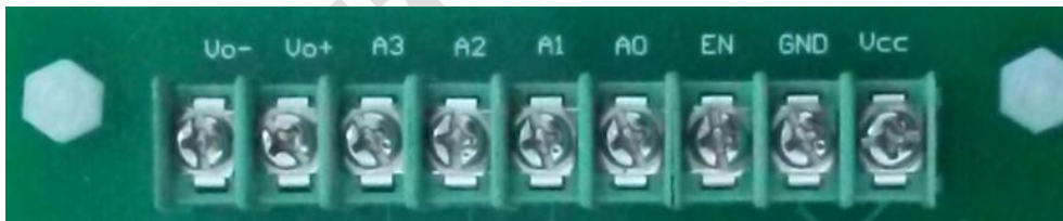
Fig2 terminals of watermeter DEMO
